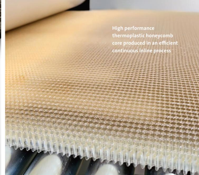
High performance thermoplastic honeycomb core produced in an efficient continuous inline process
