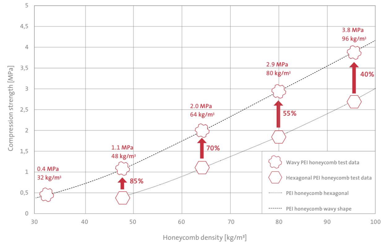
ThermHex<sup>WAVY</sup> PEI honeycomb core is a continuously produced thermoplastic honeycomb core with exceptional fire resistance and temperature stability.
